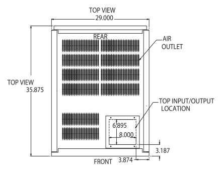
NO CLEARANCE REQUIRED ON LEFT SIDE OF UNIT OPTIONAL 12" CLEARANCE ON RIGHT SIDE OF UNIT (IF USING OPTIONAL SIDE OUTPUT TERMINATION)
