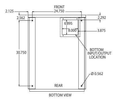
NO CLEARANCE REQUIRED ON LEFT SIDE OF UNIT OPTIONAL 12" CLEARANCE ON RIGHT SIDE OF UNIT (IF USING OPTIONAL SIDE OUTPUT TERMINATION)
